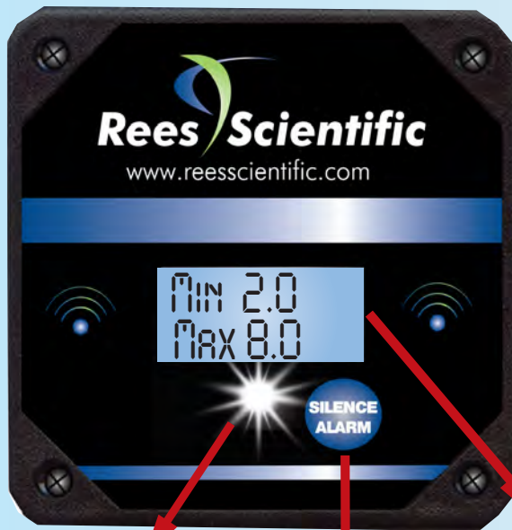
Visual Alarm Button to Inhibit Local Alarm
