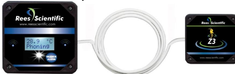
Expansion Modules with Z3 Wireless and LCD
