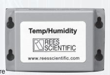
and relative humidity data are read from the digital temperature sensor and the relative humidity sensors. This information is combined with a CRC-16 error check and transmitted in a very short data packet that results in a transmitter on time of only 15 milliseconds. This architecture allows the Sensor to consume very low energy resulting in a battery life of up to 3 years.
