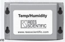
and relative humidity data are read from the digital temperature sensor and the relative humidity sensors. This information is combined with a CRC-16 error check and transmitted in a very short data packet that results in a transmitter on time of only 15 milliseconds. This architecture allows the Sensor to consume very low energy resulting in a battery life of up to 3 years.
